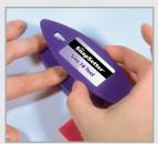
Slide the Tool Top over the post onto the Middle Positioning Bar.
