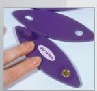
Place the Tool Base on a firm surface. With prongs facing up, place the Snap Top (A) in the indented area of the Tool Base.
