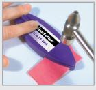
Hammer the snap parts into place on a firm surface, such as marble or steel.
